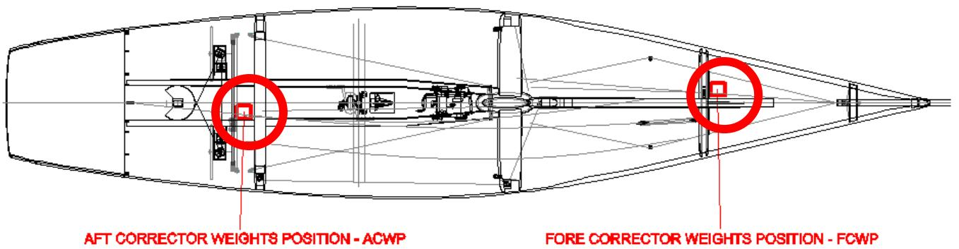
The pair(s) of corrector weights calculated in accordance with rule C.7.3 shall be positioned and permanently fastened to the liner.
